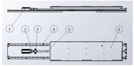
FIGURE 4: Emptying platform diagrammatic drawing2 Shaft coupling3 Ball screw block5 Ball bearing lead screw6 Platform
