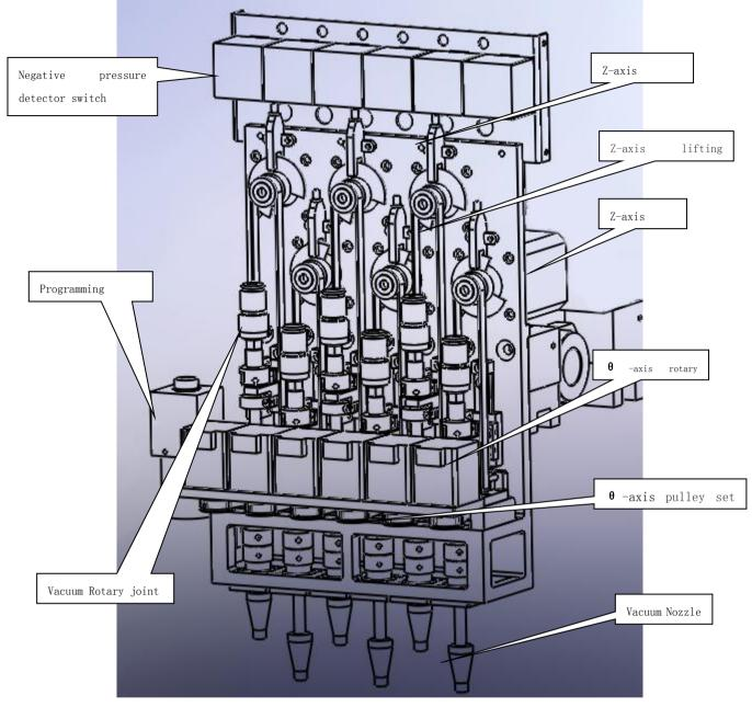
FIGURE 6: Z- Axis construction diagrammatic drawing
