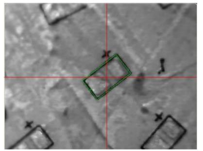
As shown above, locate the point on the bonding pad, check the image display area to make sure the image on the center, adjust the positioning frame (green box) size to match the pad of component. Drag the green box with the mouse to have the minus sign of the box to match the negative direction of the pad, select the suction nozzle and feeder and then add this point location.
