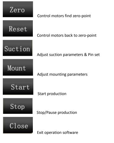
FIGURE 1 Programming options for normal PCB
