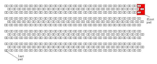
This is a four pin board, there are 84 LED chips each single board. It can be programmed as a unit for the 3 LED chips (like in the red area), add first 3 points location from top to bottom. Then take the undermost point as the "**First Pad**" of the matrix setting. 84 LED chips each single board would be 28 units in Column and 4 units in Row when setting. The setting for matrix is as below:
